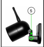
6. Adjust the angle of the camera for a desired view.
